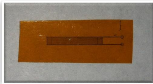
Temperature sensor printed with carbon nanotubes
