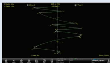
Using color bars a bending of the Green Magenta transition can indicate an inter-channel timing error within a specific component of the signal.
