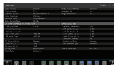
When Dolby Digital or Digital Plus is decode information on the Data Rate, Channel & Bitstream Modes are displayed. Along with the metadata parameters for Dialogue Level, Dynamic Range and Downmix.
