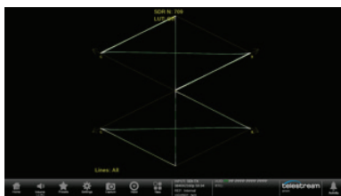
Diamond display for monitoring of RGB component signal for Camera Shading and Editors/Colorist with 100% color bars applied
