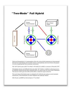
This alternate variety of the "Full" hybrid is a configuration known as "Two-Mode". It adds another power-split-device for electric motor and engine interaction, plus multiple clutches.
