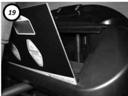
19 Carefully place the membrane in the control panel Pod (don't scratch plastic edges) tilting it towards you so you can make all connections.
