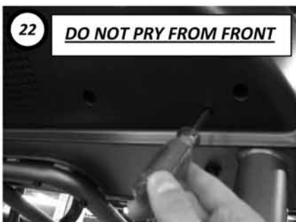
Press membrane into set position. If you need to free the membrane, use a long screw driver to pop it out from back using the access hole.
