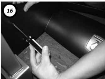
16 Install the Front Cover using 12 phillips screws (I) to secure it.
