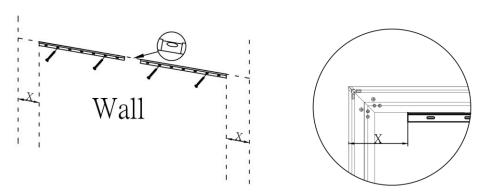
**Step 15**: Position the fixed frame screen onto the top wall brackets as shown below and push down at the center of the top of the frame to secure.
