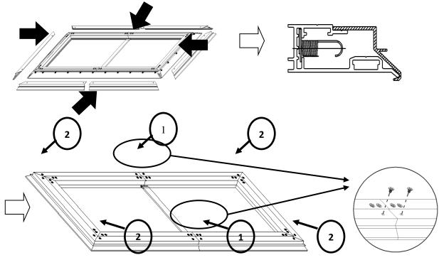
**Step 13**: Install the *angle cover* (*j*) on each corner of the frame and install the M4x7 screws to hold down the angle cover.
