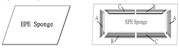
**Step 3**: Remove the foam in all frame ends before assembling the frame.
