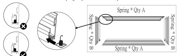
Note: The springs are pre-installed into the grooves of the frame.
