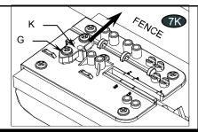
**Step 7K** - This step is for installing Splitter/ Kerf Keeper Combo only—continue to Step 8 after this step.
