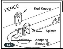
**Step 14K** - This step is for installing the Splitter/ Kerf Keeper Combo only—continued from Step 13.
