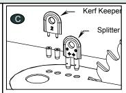
(C) An MJ Splitter Steel PRO and Kerf Keeper Combination installation is designed for solid wood ripping. This is a completely separate installation from the Double MJ PRO Splitter installation—the hole alignment is different.
