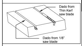
WARNING: MAKE SURE THAT YOU HAVE THE CORRECT MODEL OF MJ SPLITTER STEEL PRO SYSTEM FOR YOUR SAW BLADE PRIOR TO INSTALLATION. INCORRECTLY USING A THIN KERF SAW BLADE WITH A 1/8" SPLITTER WILL CAUSE BINDING AND DAMAGE THE 1/8" SPLITTER. USE OF THE WRONG MODEL MAY CAUSE INACCURATE ALIGNMENT, BINDING AND JAMMING.
