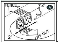
(A) With a **Double** MJ Splitter Steel PRO installation, both sides of the work piece are kept away from the spinning saw blade upon exit. This set-up works best with dimensionally stable material, e.g., plywood, MDF, etc. A minimum space of 2" is required.
