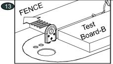
Step 13 - In the first set of mounting holes, test both surfaces of each MJ PRO Splitter facing the rip fence with Test Board-B and select the surface that best suits your preference. When cutting material other than wood, such as aluminum or plastic, use the surface that provides no tension.
