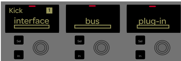
Channel Controls displays showing available input types
