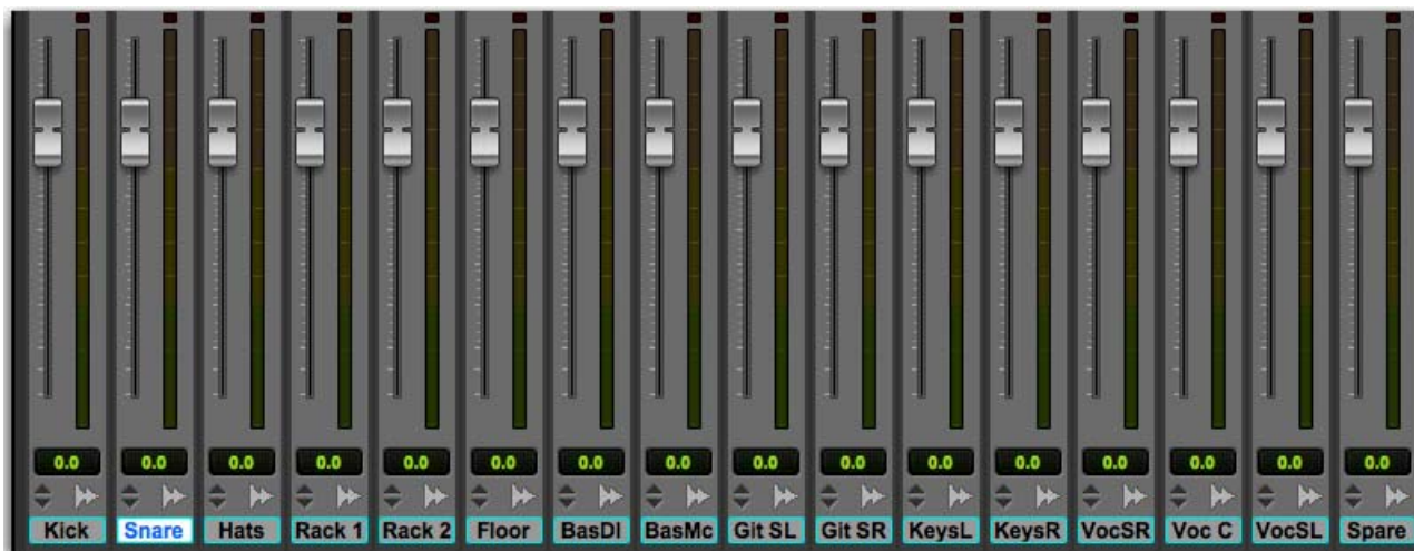
Pro Tools Mix window showing tracks currently banked to the S3 channel strips
