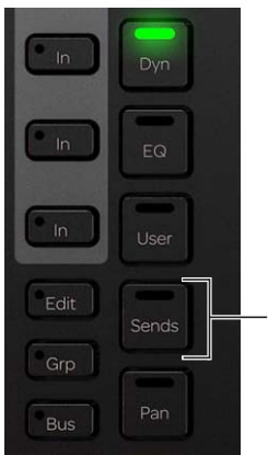
Sends switch on the Process Module
