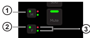
M (1) and F (2) Automation Punch (2) switches with Automation Status indicators (3)
