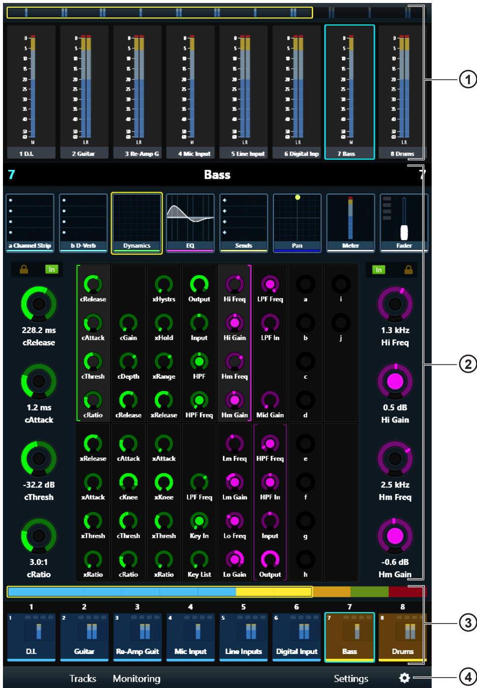
Figure 80. Home screen with Meter Scroller (1), Attention Track Editor (2), Track Scroller (3), and Home Screen Local Options icon (4)
