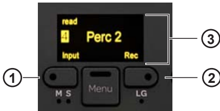
Input (1) and Record (2) switches, OLED (3)
