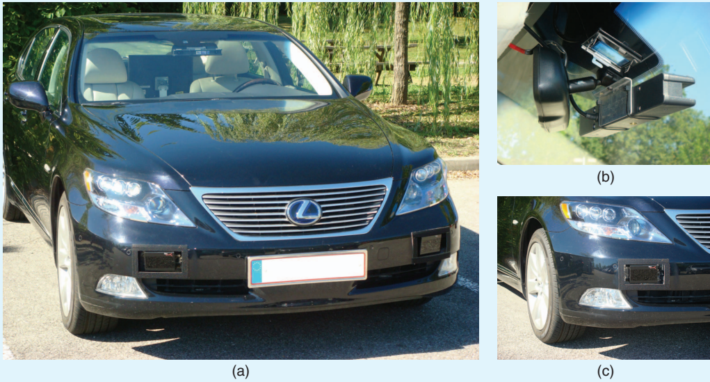
FIG 10 (a) Lexus LS600h car equipped with two IBEO Lux lidars, (b) a TYZX stereo camera, and (c) an Xsens MTi-G inertial sensor with GPS.
