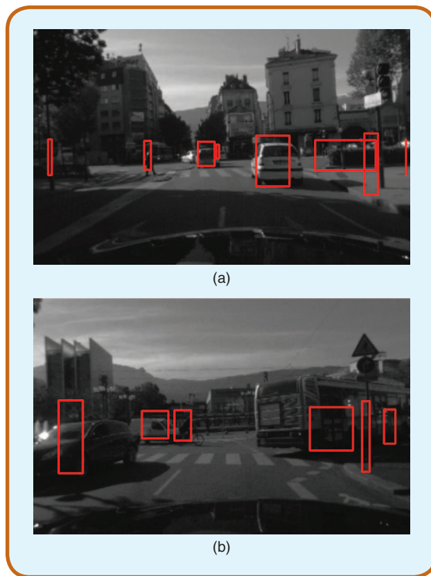
FIG 12 Example of the objects detected using BOF and FCTA: (a) cars and a pedestrian, (b) cars, a bicycle and a bus.
