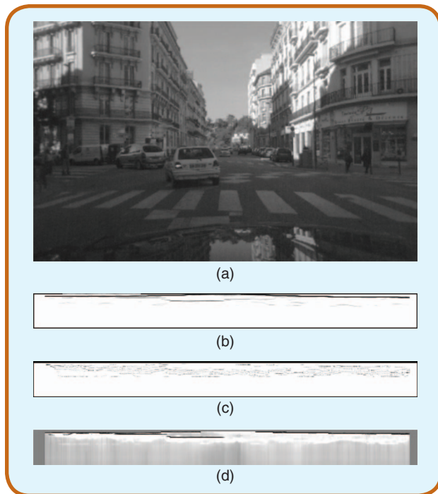
FIG 3 Computation of the occupancy grid in the u-disparity plane: (a) left image from the stereo camera, (b) obstacle u-disparity image, (c) road u-disparity image, (d) occupancy grid in the u-disparity plane.
