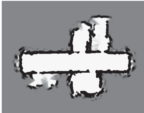
Figure 9.5 Occupancy probability map of an office environment built from sonar measurements. Courtesy of Cyrill Stachniss, University of Freiburg.
