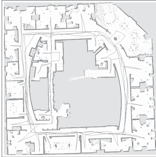
Figure 13.19 Occupancy grid map corresponding to the particle with the highest accumulated importance weight obtained by the algorithm listed in Table 13.4 from the data depicted in Figure 13.18. The number of particles to create this experiment was 500. Also depicted in this image is the path represented by the particle with the maximum accumulated importance weight.
