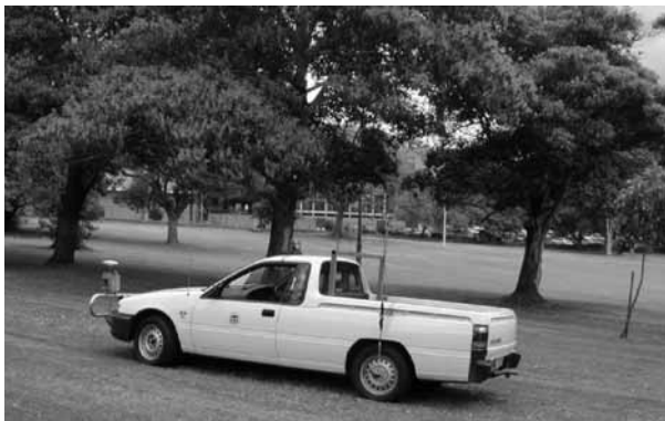
Figure 12.13 The vehicle used in our experiments is equipped with a 2-D laser range finder and a differential GPS system. The vehicle’s ego-motion is measured by a linear variable differential transformer sensor for the steering, and a wheel-mounted velocity encoder. In the background, the Victoria Park test environment can be seen. Image courtesy of José Guivant and Eduardo Nebot, Australian Centre for Field Robotics.
