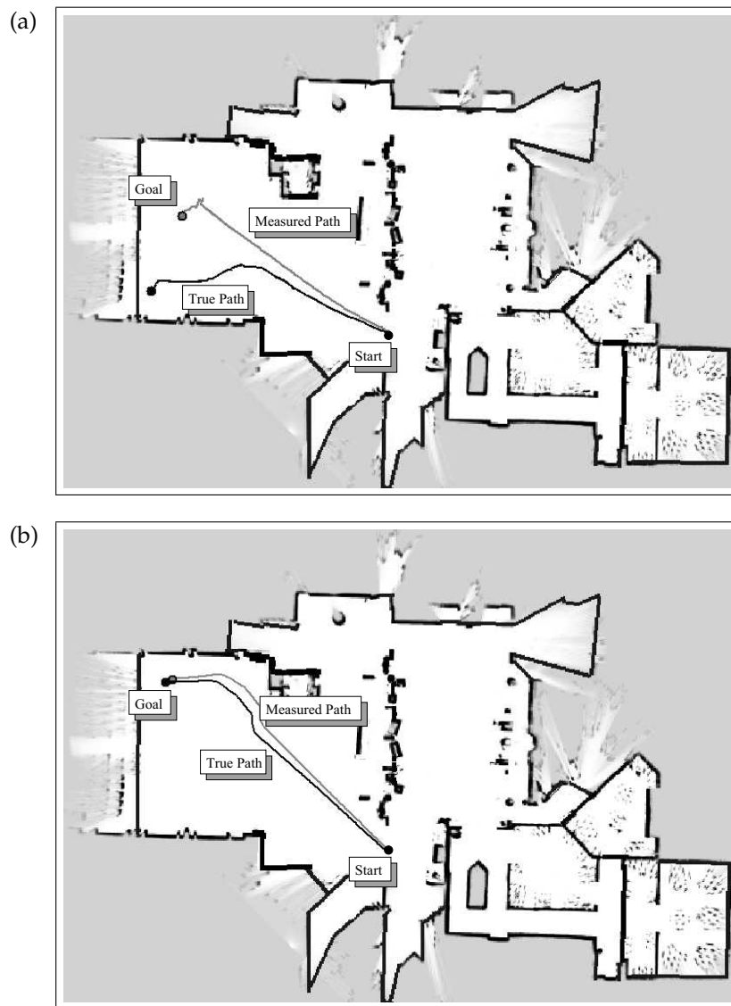
Figure 1.2 Top image: a robot navigating through open, featureless space may lose track of where it is. Bottom: This can be avoided by staying near known obstacles. These figures are results of an algorithm called coastal navigation , which will be discussed in Chapter 16. Images courtesy of Nicholas Roy, MIT.
