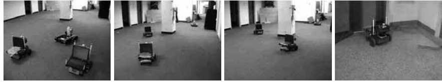
Figure 17.11 Coordinated exploration by a team of mobile robots. The robots distribute themselves throughout the environment.
