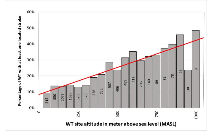
Clear trend of increasing probability of upward lightning to WT with increasing altitude of installation site above sea level
