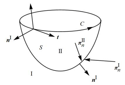
In this figure,  $\mathbf{t}$  is a unit vector tangential to the bounding curve C at every point. The direction of the force due to surface tension is then  $\mathbf{n}^{\mathrm{I}} \times \mathbf{t}$ . The subscript n is included on the stress tensors to indicate that the forces (per unit area) are acting on a surface whose normal unit vector is  $\mathbf{n}^{\mathrm{I}}$ . Newton's second law becomes
