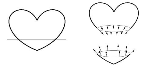
This figure illustrates the forces due to surface tension in one cross-section of the boundary. As  $\sigma$  has units of force per unit length, the total force due to surface tension is obtained by integrating  $\sigma$  over the bounding curve C.
