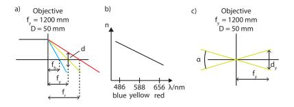
Aberrations in the optics will degrade the image. A "commercially available ocular" implies that all aberrations have been minimized in the ocular. Therefore, all aberrations in the image will come from the objective.
