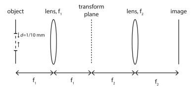
A typical Fourier optical arrangement is shown in the figure above. The transform plane is the Fraunhofer diffraction pattern of the object. We want to construct a filter which absorbs the diffraction pattern from a perfect wire grid. Any errors in the grid will change the diffraction pattern so that some light is transmitted through the filter, reaching the image plane. If a detector is placed in the image plane, any signal will then correspond to a faulty grid.
