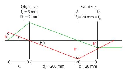
The Huygens eyepiece has a field lens with the same focal length as the eye lens. The distance between the lenses is the same as the focal length so that the lenses are placed in each others focal planes. We have a microscope so the final image should be in infinity and the objective should be the aperture stop (AS). From the green ray figure
