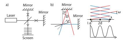
Turning the mirror slightly will change the angle between the wavefronts (figure b). This will give fringes with a period of
