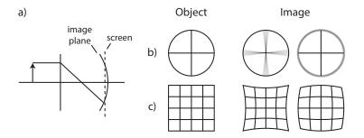
a) The image plane is bent  $\rightarrow$  Field curvature
