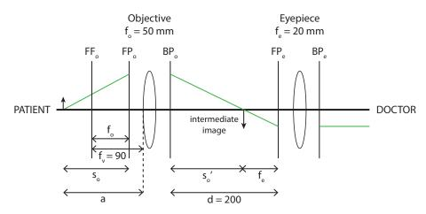
We have a microscope so we want the final image to be in infinity. Combining that with the information in the text gives a system like the one in the figure above.
