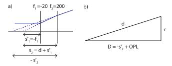
The laser is imaged through the lens system (figure a). The final image of the laser after the second lens is located at
