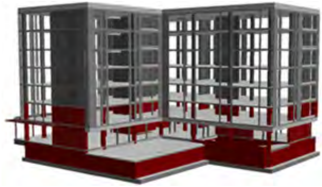
Fig. 6. The example building as an example for avoiding torsionally flexible system
