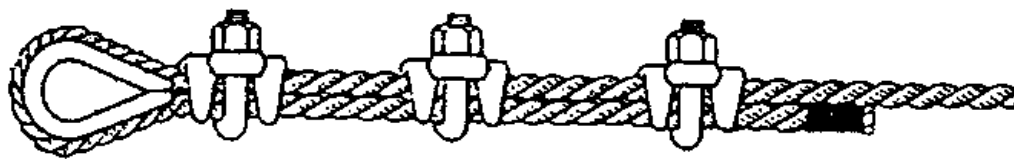
RIGHT WAY FOR MAXIMUM ROPE STRENGTH
