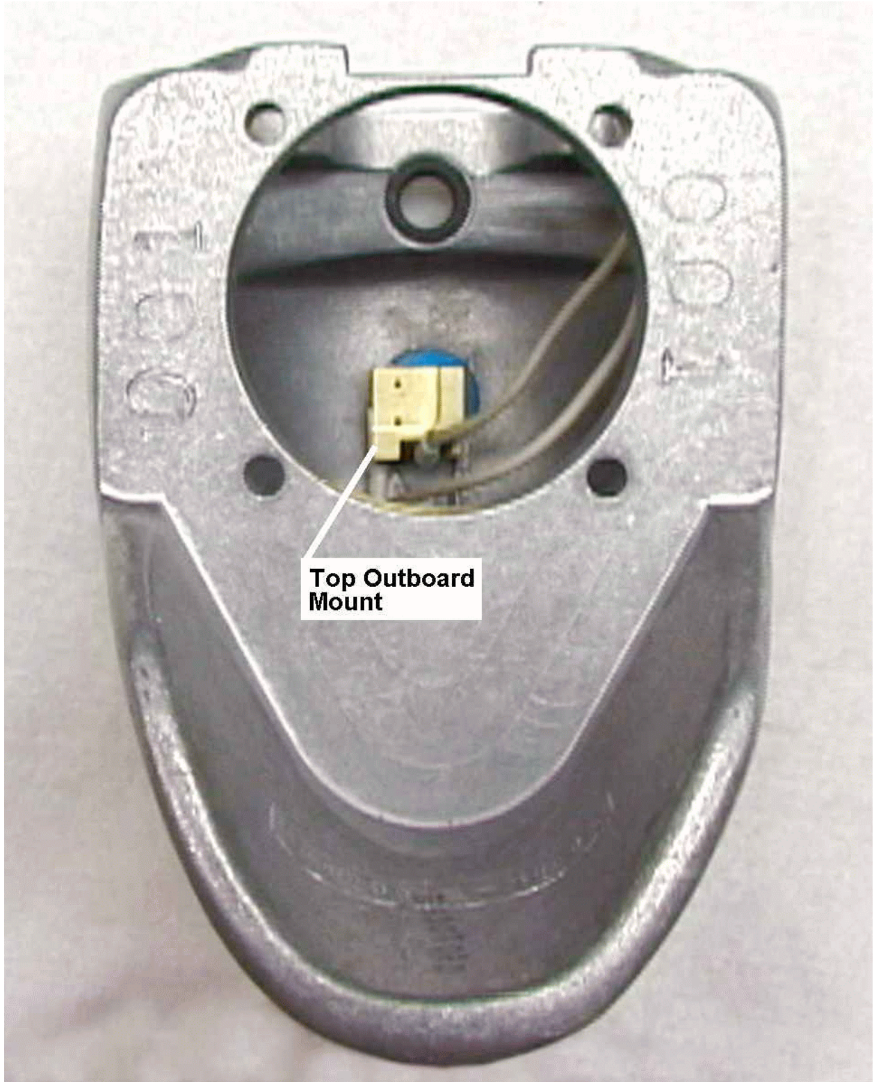
Figure 3.3 -- Bottom view of accelerometers on top outboard mount installed in skull
