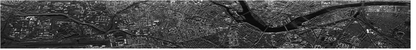
Fig. 11. High resolution acquisition example: X-band acquisition of downtown Toulouse from a C160-Transall aircraft. Bandwidth is 1.224 GHz (5 successive frequency agilities covering 240 MHz each), duration is 120 s, signal size (single channel 8 bits) is 34.3 Gb, full resolution swath is 1200 m (slant), stripe length (for square resolution) is 9300 m.
