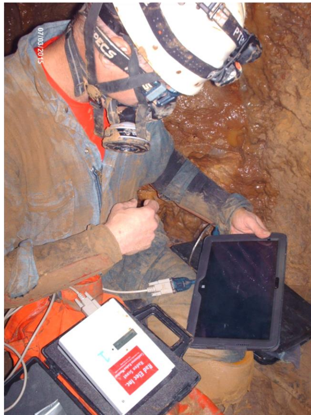
Figure (4): Using a tablet computer to launch the RSP in Kemling Cave.
