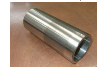
Overlay welding is used to weld Tungsten-carbide complex alloys to pump sleeves
