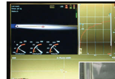
Thermal spray particle monitoring system (Accuraspray-gs manufactured by TECNAR)
