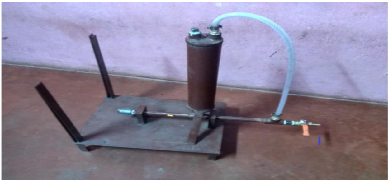
FIGURE (2): FABRICATED PORTABLE ABRASSIVE JET MACHINE
