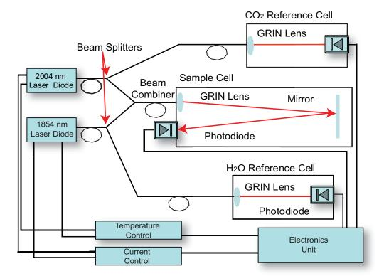
Figure 1: Dual laser TDLAS set up
