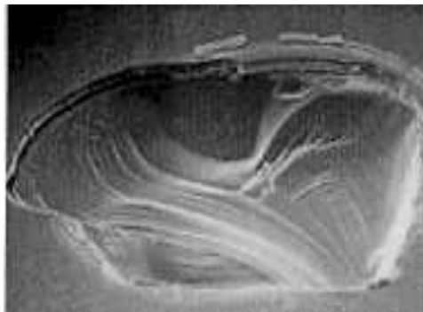
Figure 3.1.1. Cratering in silicon 1
