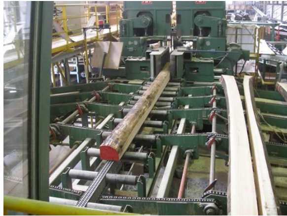
Figure 3: Quarter-sawing flitches with a slab sawing strategy at McCormack Demby Timbers, Morwell, Victoria (Source: Washusen et al. 2009d)
