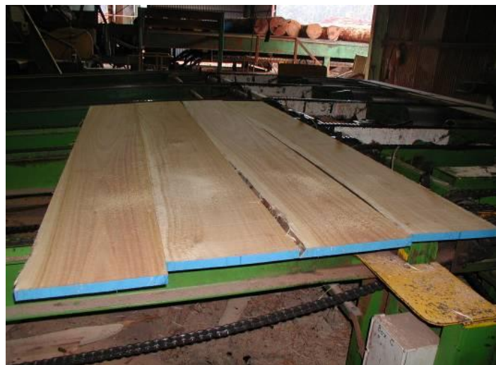
Figure 13: Slabs produced during sawing trials in thinned and pruned 22-year-old E. globulus at Auswest Timbers, Pemberton, WA. Splitting of slabs like these was rare suggesting that growth stresses did not hinder the sawing process (source: Washusen et al. 2004).
