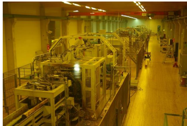
Figure 26: A HewSaw SL 250 at United Sawmills Ltd, Pori, Finland (source: Washusen 2008).
