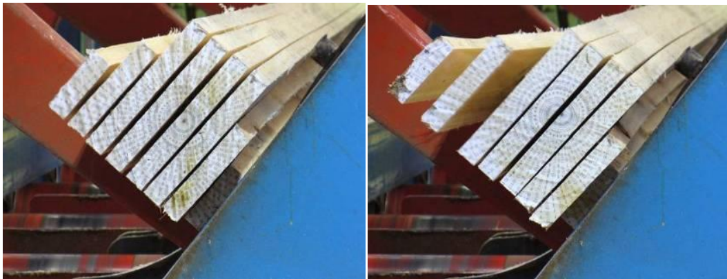
Figure 21: The approximate range in board deflection for 17-year-old Eucalyptus nitens logs observed in trials with the HewSaw R250 (source: Washusen et al. 2007b).
