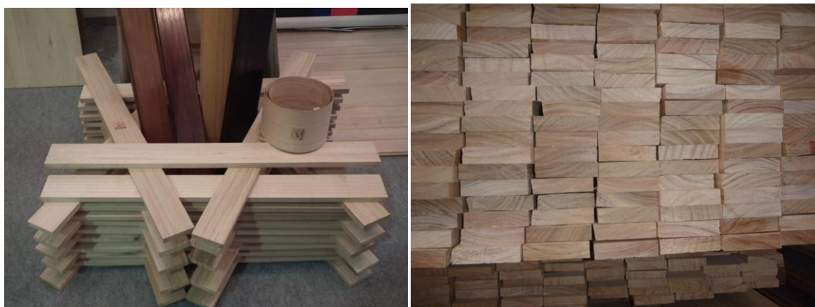
Figure 38: Thin section (12 mm) E. nitens boards and sliced veneer (left), and docked board ends showing no signs of internal checking (right). All products produced in Chile (Photo: Evan Shield).
