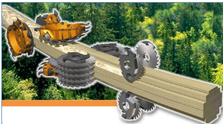
Figure 20: Diagrammatic representation of the internal arrangement of chippers and saws in the HewSaw R250 (source: www.hewsaw.com ).
