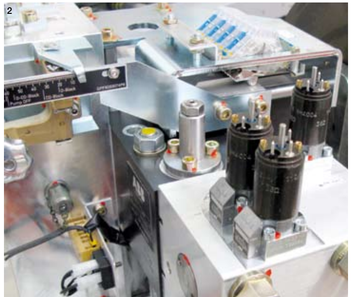
1 Circuit breaker operating mechanism of type HMB-1 | 2 Pilot valves for HMB-2 circuit breaker operating mechanism
