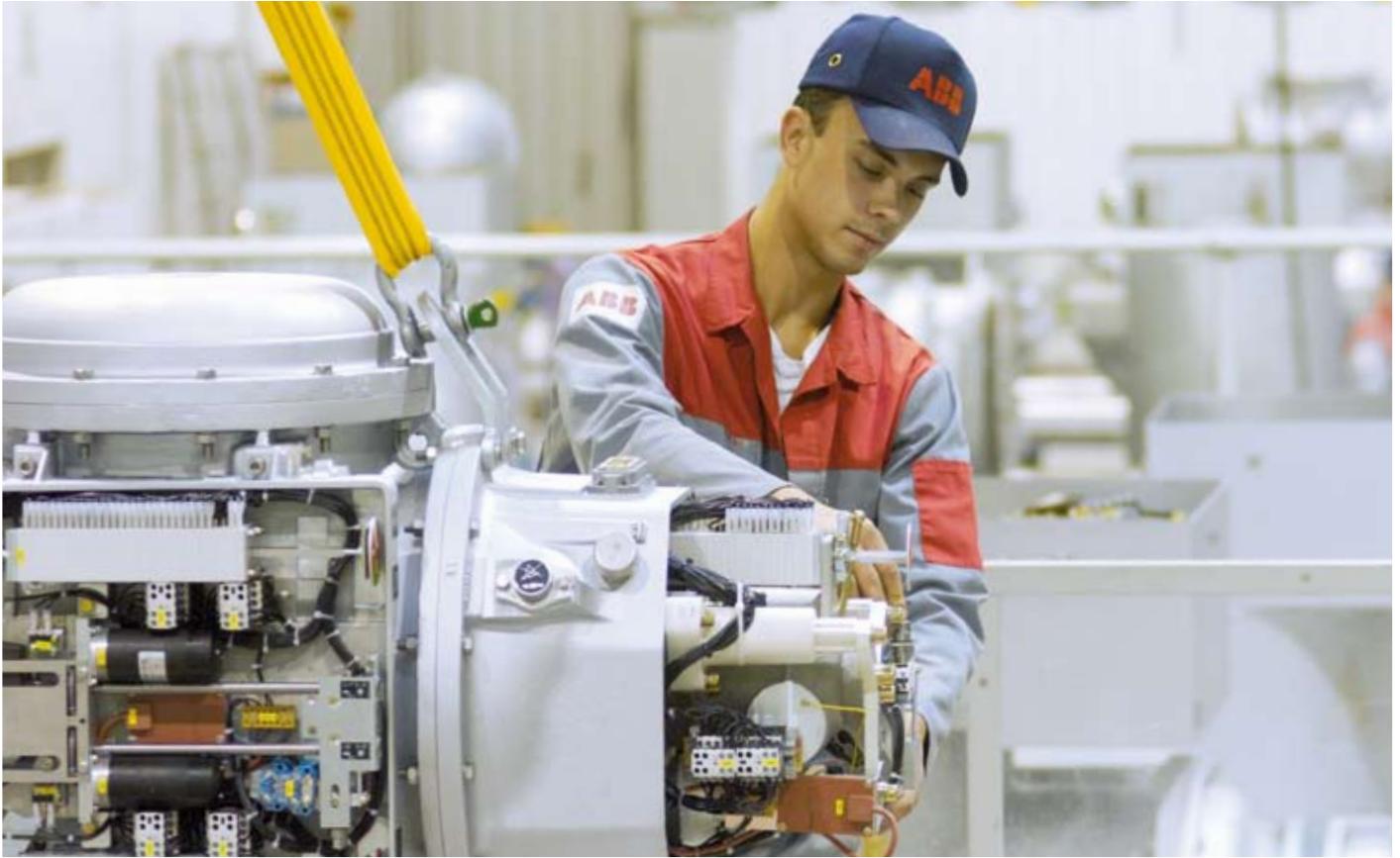
Mechanical routine test of the make-proof earthing switch
