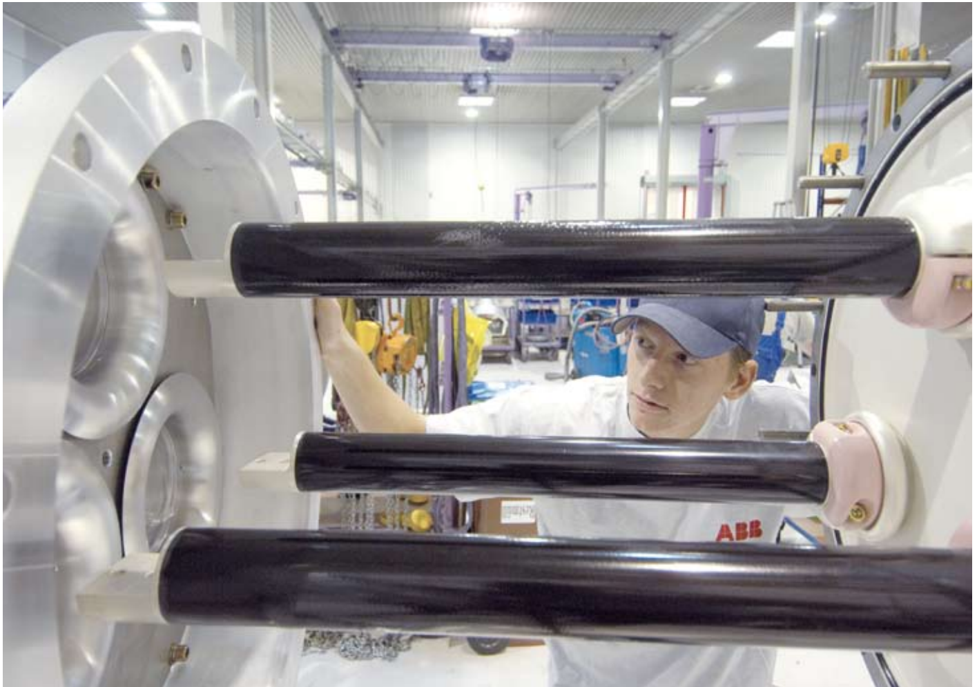
Assembly of integrated current transformer
