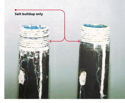
Example of hot-dip galvanized threads after 42-day salt-fog test.
