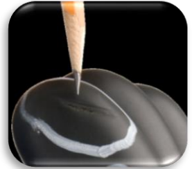
Grooves worn due to rope burns or heat exposure
