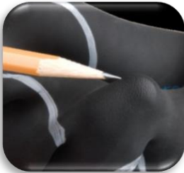
Checking for cracks due to UV or ozone
