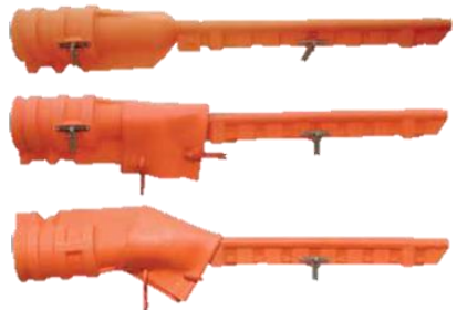
Deadend Cover couples with Conductor Cover using Hot Sticks or Rubber Gloves. (Must be used with Rubber Insulating Blanket)
