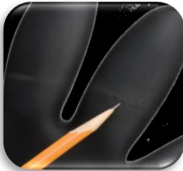
Weak creases resulting from being left too long inside out or folded
