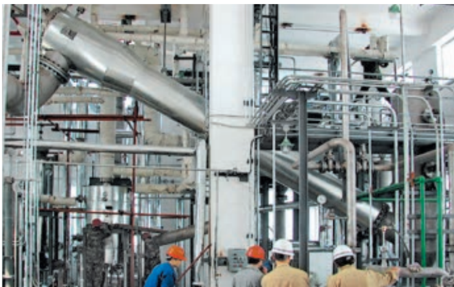
Fig. 3 3-stage steam jet vacuum pump with mixing condenser and liquid jet vacuum pump in a polyester production plant
