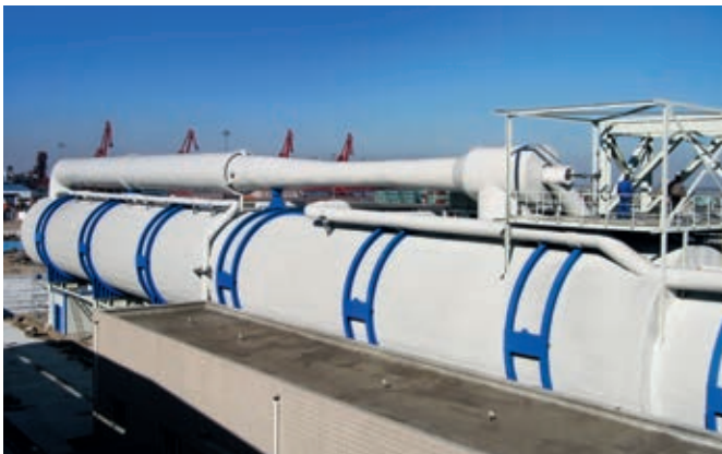
Fig. 4 Vacuum unit for a MED plant for sea water desalination with a capacity of 800 t/h of distillate
