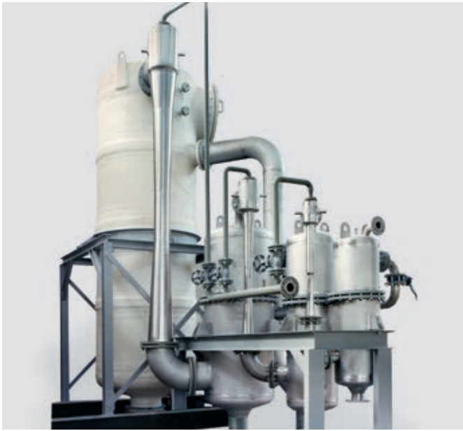
Fig. 2 3-stage steam jet vacuum pump with mixing condensers Suction capacity: 3380 kg/h steam and 225 kg/h of inert gas from 60 mbar
