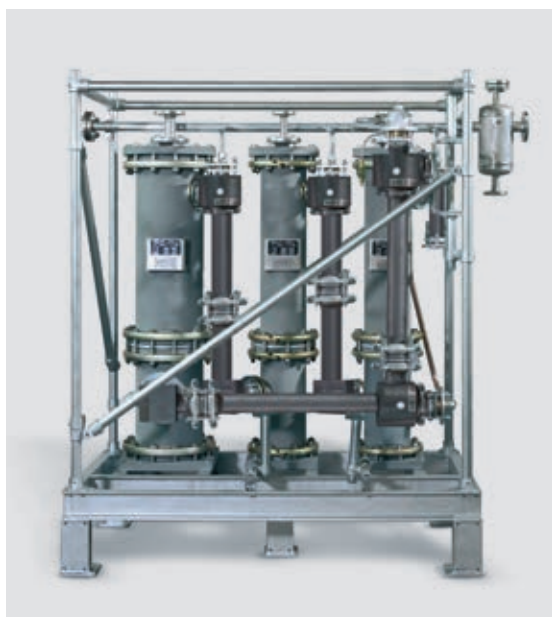
Fig. 2 5-stage steam jet vacuum pump in corrosion-resistant design Materials: jet pumps in graphite, mixing condensers in C-steel, enamelled Suction capacity: 5 kg/h of air from 2.5 mbar abs.
