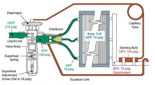
FIG. 3 -THERMAL REXPANSION VALVE (TXV) COMPONENTS
