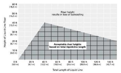
Note: Preselected liquid-line diameters independent of line length or rise, within the premissible guidelines, for properly charged RAUP units in normal air-conditioning applications.
