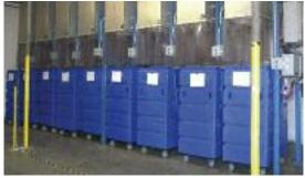
Sorting machine which is used to automatically sort linens before being washed.
