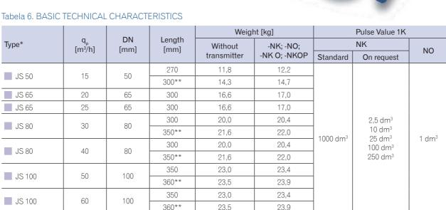
\*) - NK- pulse transmitter (Reed contact)- remote transmission of the volume indications
