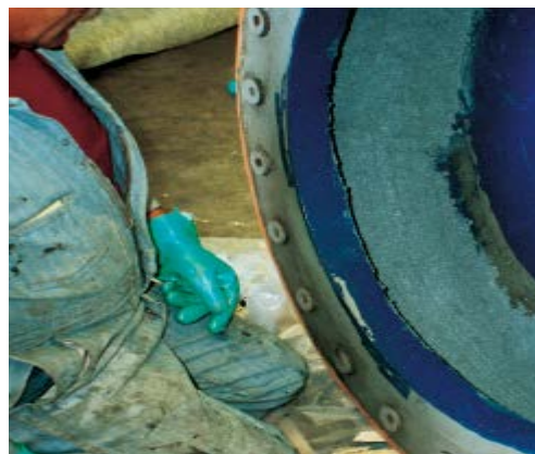
Wear Guard Fine Load offers an economical way to protect equipment surfaces from abrasion damage caused by particulate less than 3mm.
