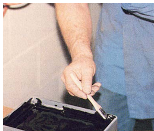
Flexane 80 Liquid is used to make a mould pattern.
