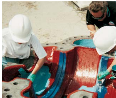
Brushable Ceramic provides pumps and other equipment with a smooth protective barrier against wear, abrasion, corrosion, erosion and chemical attack and it fills holes and voids in castings.
