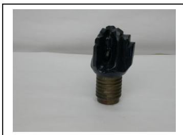
Step Type Bit with N Rod Thread
