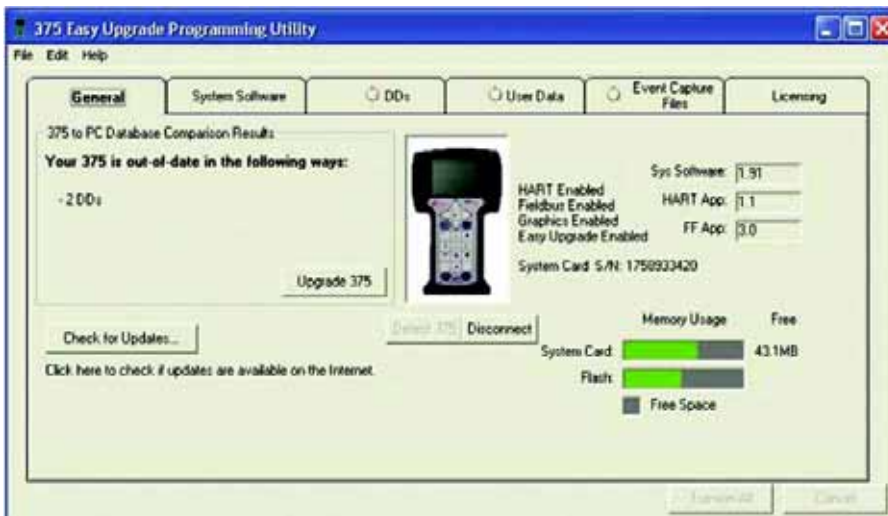
FIGURE 4. Easy Upgrade allows communication between the 375 Field Communicator and a PC using IrDA. The IrDA port enables transfer of configuration data and upgrades between the 375 and AMS Device Manager.
