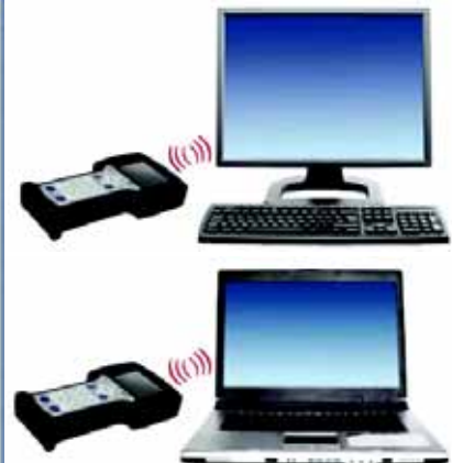
FIGURE 4. Easy Upgrade allows communication between the 375 Field Communicator and a PC using IrDA. The IrDA port enables transfer of configuration data and upgrades between the 375 and AMS Device Manager.
