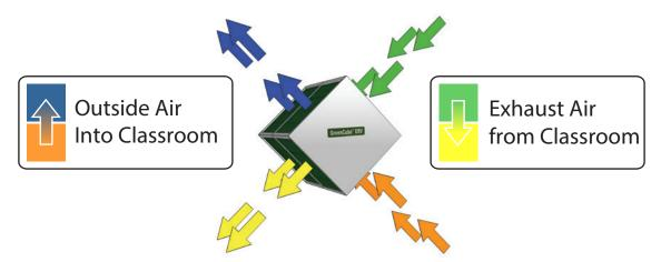
The GreenCube<sup>®</sup> ERV is only available on HVPSA units (2-stage compressor). All HVPSA units with the GreenCube<sup>®</sup> ERV, including the HVPSA36 and HVPSA42, are in the HVPSA49/60 cabinet (see page 28).
