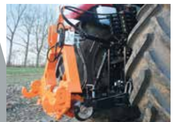
Solid adaptor frame with side-shift
