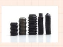
Fasten collars, sheaves, gears, knobs on shafts. Locate machine parts. Self-locking knurled cup point is standard. Special Points like Flat, Dog, Cone & Plain Cup are also available.
