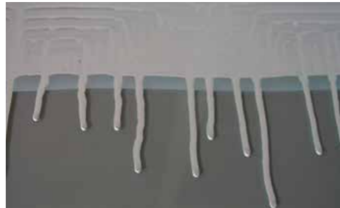
Sagging of paint on vertical substrate
