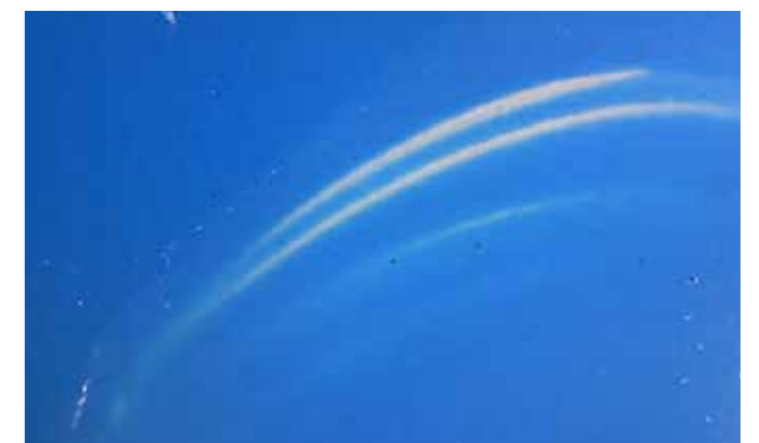
Excellent pigment stabilization "rub out test"
