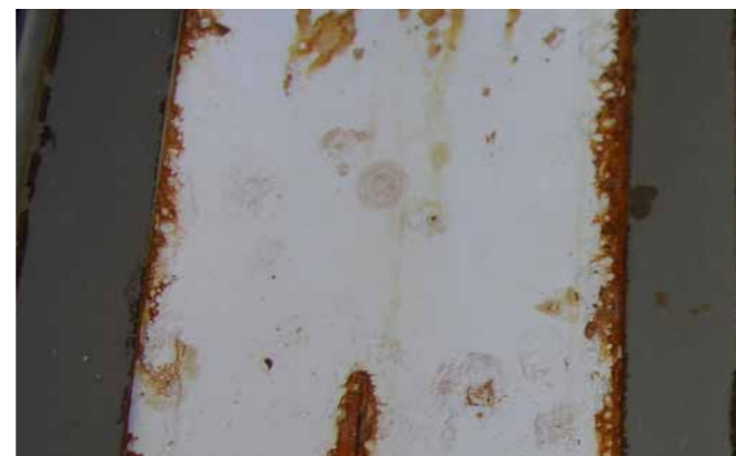
Weak corrosion protection in 2 layer system
