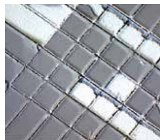
Loss of interlayer adhesion
