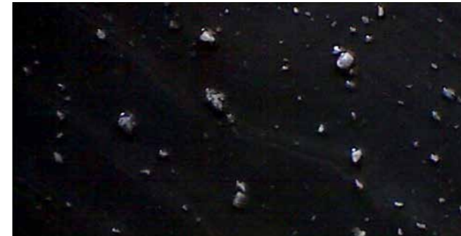
Destruction of wb Epoxy formulation by ionic dispersants
