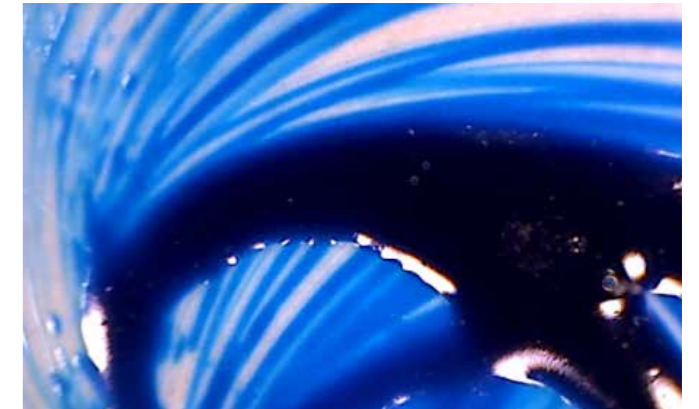
Strong pigment floating visible "rub out test"
