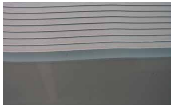
Paint stays on vertical substrate without sagging
