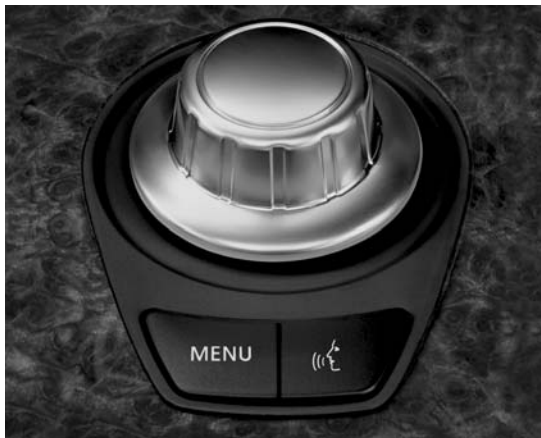
The iDrive controller is on the console behind the shift lever. Voice Command (right-hand button) is included in the option.
