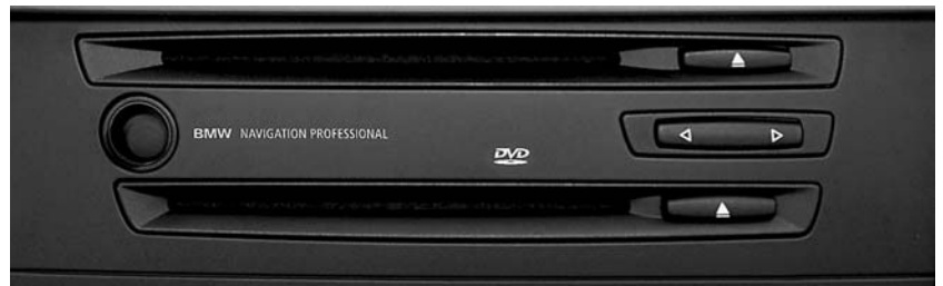
In vehicles with the Navigation/iDrive option, as shown here, hard controls are reduced and many functions appear in the iDrive control display. The two disc slots are for the standard single-disc CD player (upper) and Navigation DVD (lower).
