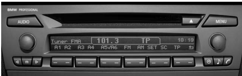
In vehicles without the Navigation/iDrive option, all audio functions are served by hard controls. The Professional audio unit, with display and controls as shown here, is standard in all models.
