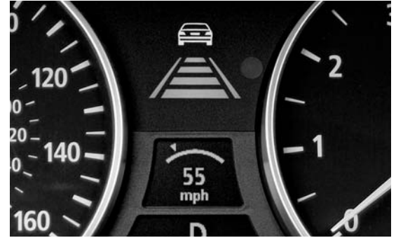
Active Cruise Control display in instrument cluster: upper graphic is for following distance, lower indication is for set speed.
