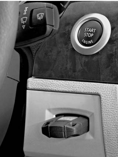
A new-type keyless remote control, similar to that of the 7 Series, inserts into a slot below the Start/Stop button.
