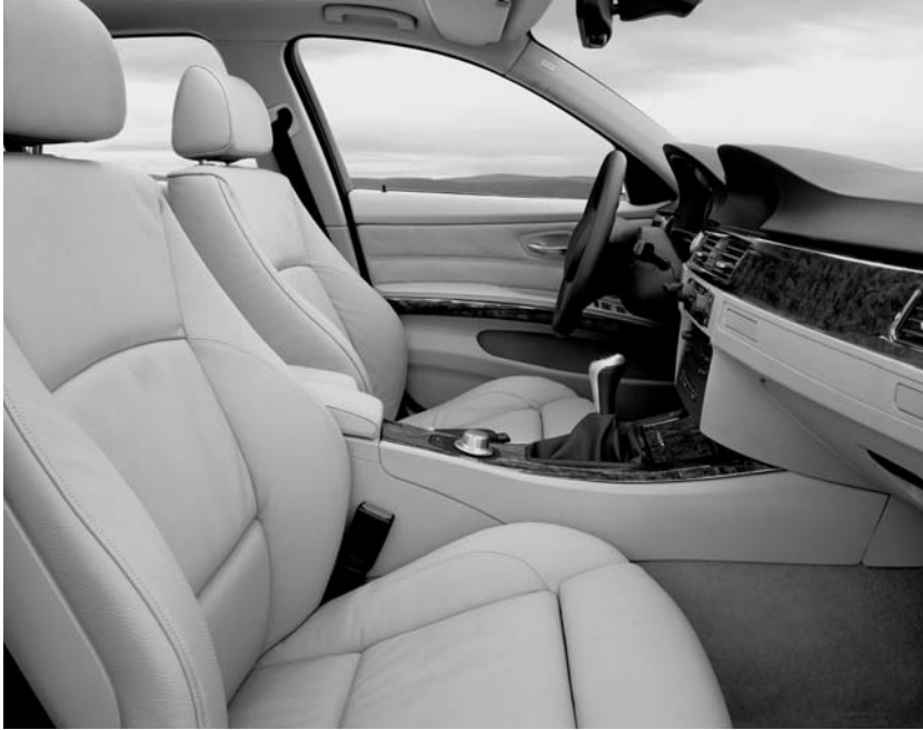
The front passenger’s door (above) includes a vertically oriented door pull. On the driver’s door, the pull is integrated into the armrest, as a vertical pull would hinder access to the power-window controls.
