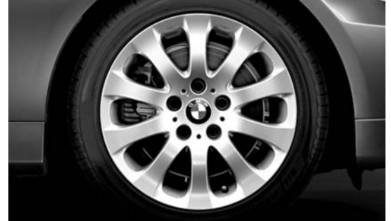
To emphasize all-season abilities, yet also add to dry-road handling and sporty appearance, the 325xi Sport Package comes with 17 x 8.0 wheels and 225/45R-17 H-rated all-season tires. The wheel design is Star Spoke #159.
