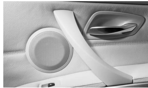
The front passenger’s door (above) includes a vertically oriented door pull. On the driver’s door, the pull is integrated into the armrest, as a vertical pull would hinder access to the power-window controls.
