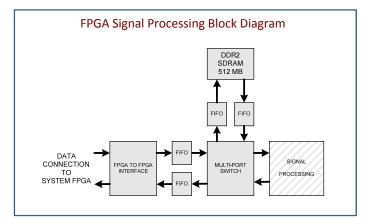
When FPGA processing is enabled, acquired data is transferred from the System FPGA to the Signal Processing FPGA where the targeted signal processing routine is conducted. The resulting processed data output is then transferred back to the System FPGA, which can then stream the resulting data to the host PC system via the PCle interface with PCle Buffered Acquisition mode.
