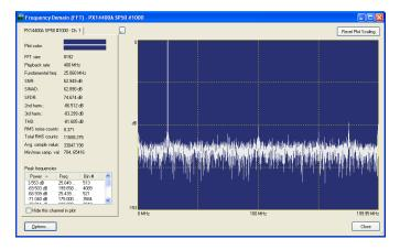
The FFT window is divided up into two regions. The left side is a tab control that contains various FFT and time-domain statistics. There is one tab for each channel of data. The right side contains the frequency domain plots of all channels.
