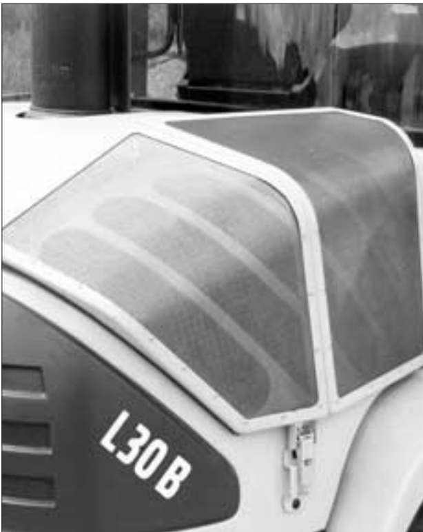
Cooling Air Filtration Screen ( 2,5 mm )
