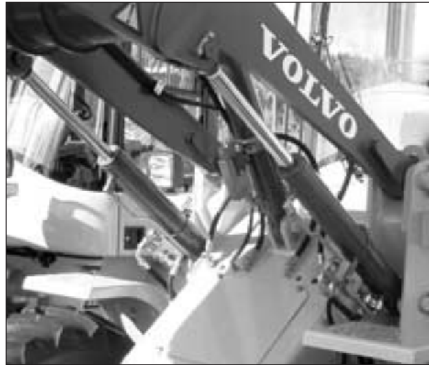
Safety Valve for Lift Cylinders
