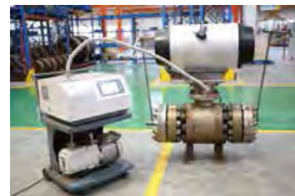
Low Fugitive Emission Test
