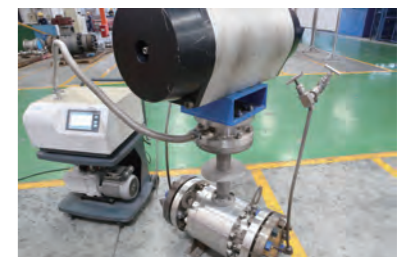
Low Fugitive Emission Test
