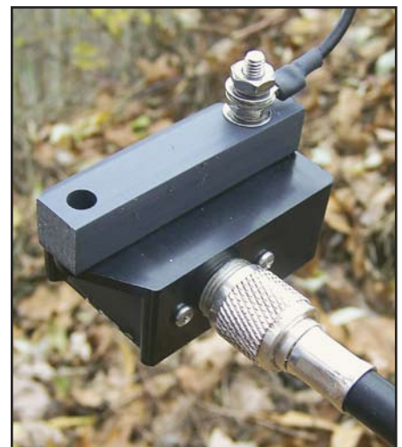
The EF-20 matching unit converts the high impedance at the end of the antenna to 50 \Omega for the transmission line.
