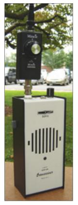
**Figure 7** — Here's the finished HT-7 with its optional Miracle Antenna tuner and whip.
