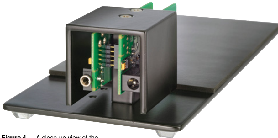
Figure 4 — A close-up view of the TP-1 showing the coaxial power jack and 1/8 inch stereo phone jack for the keyer cable.
