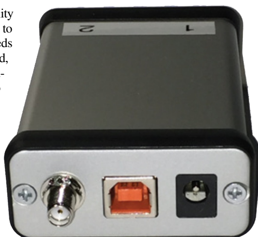
Figure 6 — One end of the enclosure has an SMA connector for a user-supplied GPS antenna, USB jack for connection to a computer for setup, and dc power jack. The two oscillator outputs are on the opposite end of the enclosure.
