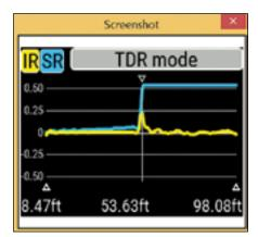
Figure 13 — Using the *AntScope* software to view the TDR measurement of Figure 12.
