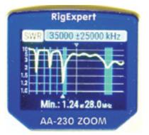
Figure 9 — A 10 – 60 MHz scan of the author's TH1 antenna. Note that the frequency of minimum SWR is indicated.
