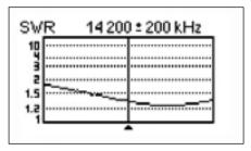
Figure 3 — Measured SWR of the EFHW-8010-1K in the reviewer's station across 20 meters. This is fairly typical of what we observed.
