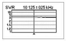
Figure 5 — Measured SWR of the EFHW-8010 in the reviewer's station across 30 meters. This was the band with the worst SWR, and still likely within the range of "trimming" type antenna tuners.
