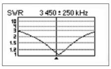
Figure 7 — Measured SWR of the EFHW-8010 in the reviewer's station with the antenna analyzer centered below the bottom of 80 meters. This is indicative of how the antenna would operate over 80 meters if it were shortened to move its resonance to mid band.
