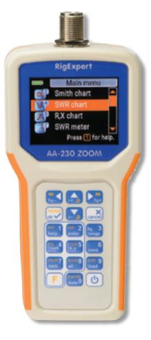
square wave rich in harmonics, however, so this must be considered when making measurements. The AA-230 ZOOM can zero out a transmission line for making accurate remote antenna feed point impedance measurements if calibration standards are available.<sup>1</sup>
