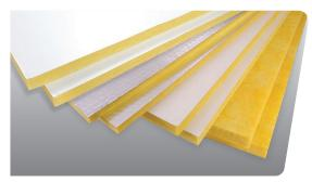
800 Series Spin-Glas® is a fiberglass equipment and external duct insulation offered in a variety of different densities. The board is available plain or with a vapor-retarder FSK, AP, or Ultra (poly-top) facing. The insulation can be readily cut with a knife and secured in place with mechanical fasteners and/or adhesives.
