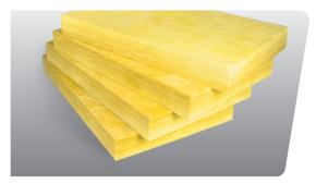
Fabrication Board is a fiberglass insulation that is designed to be used to fabricate custom pipe and tank insulation in routine commercial and industrial heating and process equipment applications. Fabrication board is light, strong, and resilient for easy fabrication and installation, and it is available in two densities with two different temperature ratings. Typical applications include pipe and tank insulation.
