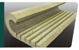
MinWool-1200 Field-Formed Pipe insulation is made of inorganic fibers derived from basalt, a volcanic rock. It is made with a thermosetting resin binder. Field-Formed Pipe insulation is a factory "V-grooved" mineral wool board with a unique contact adhesive in the grooves. It is manufactured to specific pipe sizes with a variety of facing options. It ships flat and allows for easy forming at the job site.
