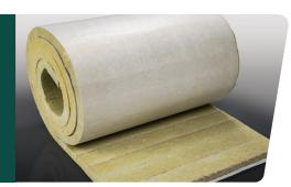
MinWool-1200 Lamella Tank Wrap is a flexible mineral wool wrap insulation. It is a lightweight, high-performance insulation for high-temperature applications. This insulation is produced to fit large diameter pipe, duct, tanks and equipment, ranging in temperatures from below ambient up to 1000°F continuous maximum service temperature.
