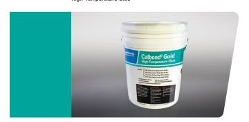
CalBond Gold is a modified, silicate-based glue for thermal insulations. It sets quickly to provide a high-temperature bond for porous insulating materials. CalBond Gold is useful for bonding sections of calcium silicate or perlite high-temperature pipe or block insulation and to make mitered elbows, large insulating sections or other special shapes.
