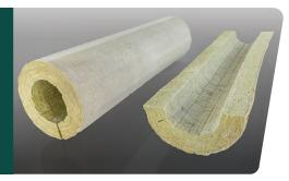
MinWool-1200 Preformed (PF) Pipe insulation is made of inorganic fibers derived from basalt, a volcanic rock. It is made with a thermosetting resin binder. PF Pipe insulation is a factory "V-grooved" mineral wool board that is formed to specific pipe sizes and provided in half cylinder sections with a variety of facing options.
