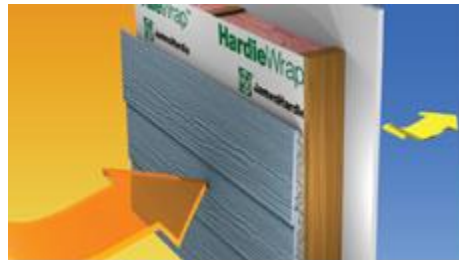
Figure 22: Hardi Plank Lap Siding with Insulation
