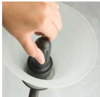
Fit bottom (open end) of socket collar tool over socket ring. Twist right until tight.
