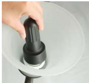
Hold socket collar tool by narrow end, open end facing down over socket ring
