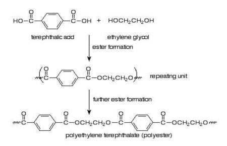
Figure 2: Mechanism of preparation of Polyester.
