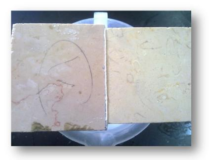
Figure 16: The sample after soaking in Water.
