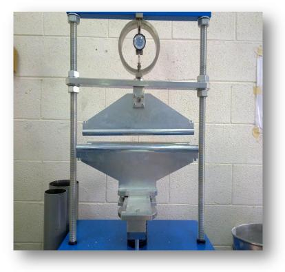
Figure 8: Flexural machine.
