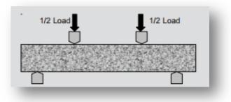
Figure 7: 4-point flexure test.
