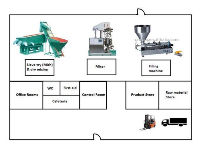
Figure 23: The lay out of the plant.
