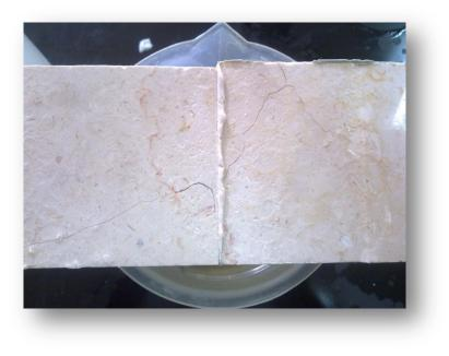
Figure 15: The sample after soaking in HCl.
